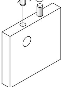
Apply glue on all wooden dowels to ensure integrity of the structure.
