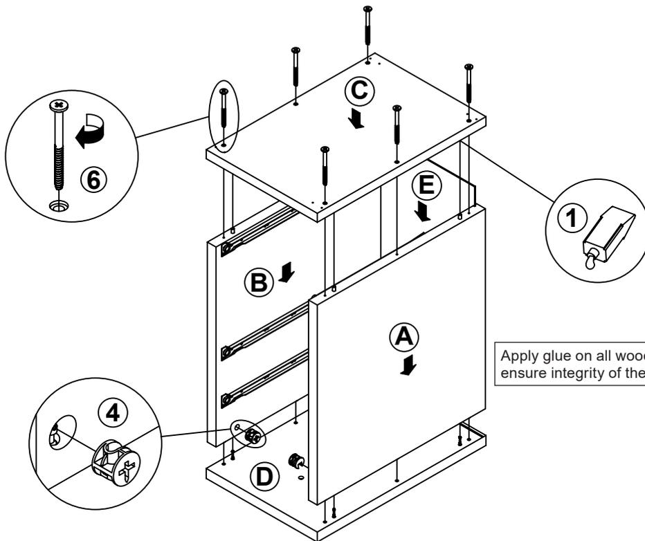
Apply glue on all wooden dowels to ensure integrity of the structure.
