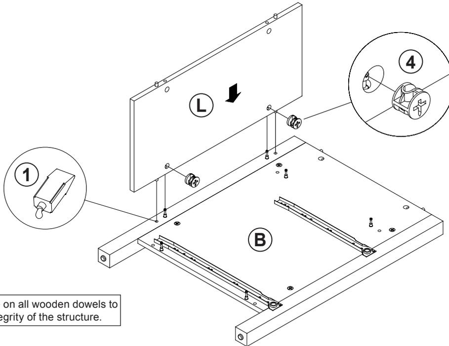
Apply glue on all wooden dowels to ensure integrity of the structure.
