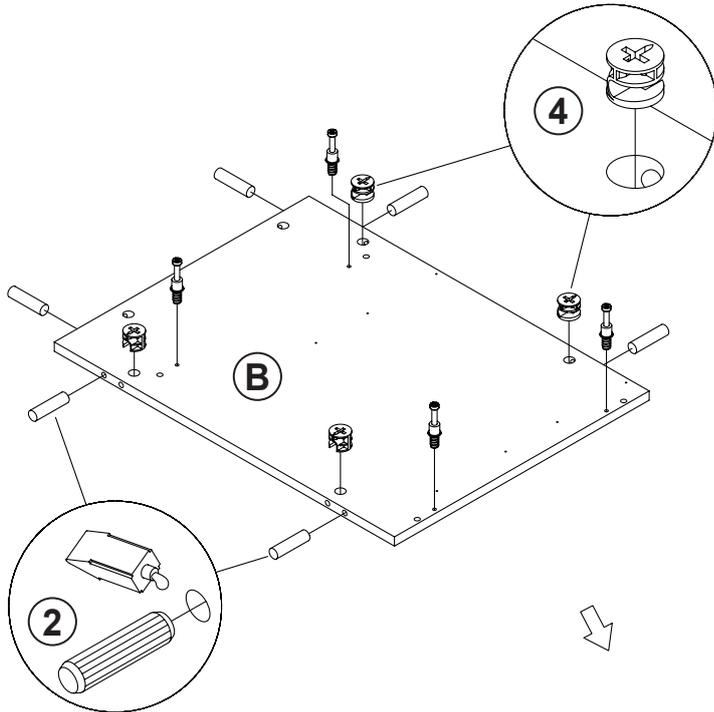
Apply glue on all wooden dowels to ensure integrity of the structure.
