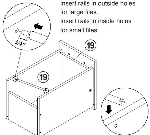
Insert rails in outside holes for large files.
