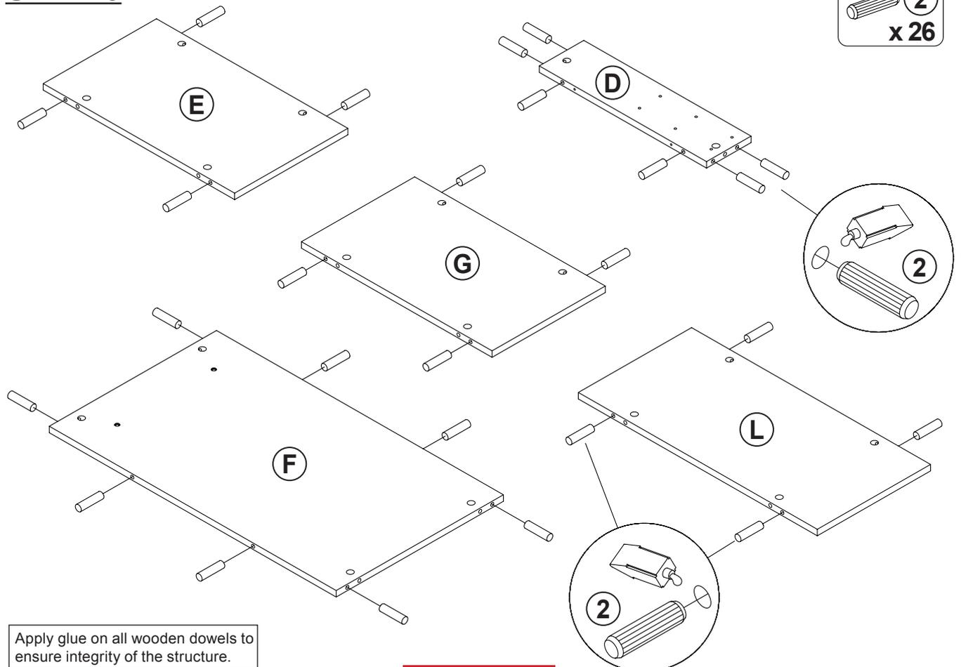
Apply glue on all wooden dowels to ensure integrity of the structure.
