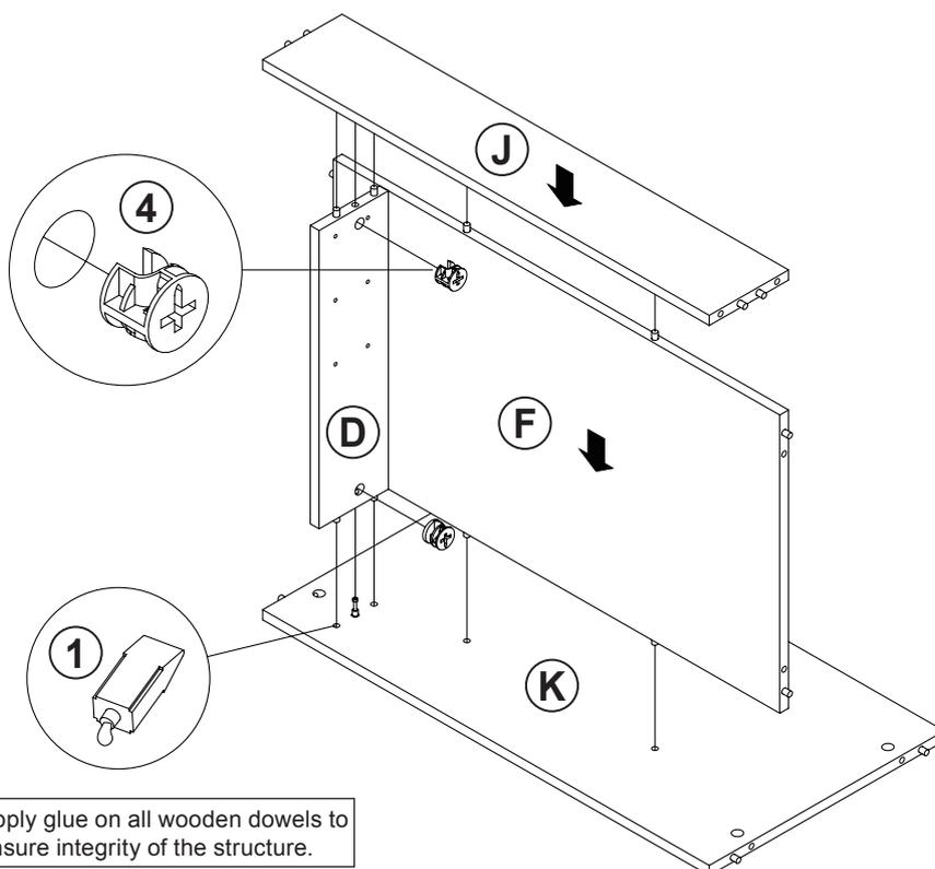
Apply glue on all wooden dowels to ensure integrity of the structure.
