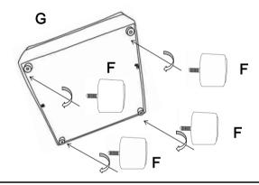
STEP 7 Please remove the wood block with screwdriver, do not use a hammer
