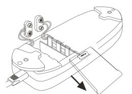
**Step 1**.Unplug the external transformer power cord from the electrical outlet. And open the marked battery door on the external transformer.
