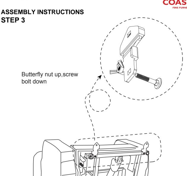
Find a small bag in the accessories box. Take out **Antifall Brackets\*2(D)** from the small bag. Assemble the two Anti-fall Brackets as shown on the bottom of mechanism to avoid toppling and falling.
