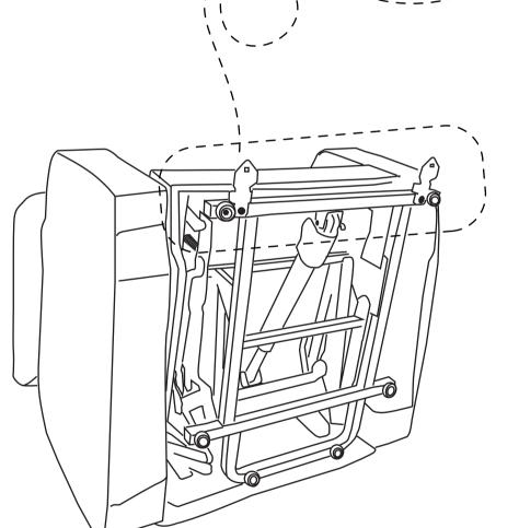
Find a small bag in the accessories box. Take out **Antifall Brackets\*2(D)** from the small bag. Assemble the two Anti-fall Brackets as shown on the bottom of mechanism to avoid toppling and falling.
