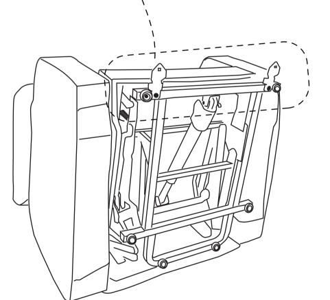
Find a small bag in the accessories box. Take out **Antifall Brackets\*2(D)** from the small bag. Assemble the two Anti-fall Brackets as shown on the bottom of mechanism to avoid toppling and falling.
