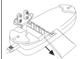
**Step 1**.Unplug the external transformer power cord from the electrical outlet. And open the marked battery door on the external transformer.
