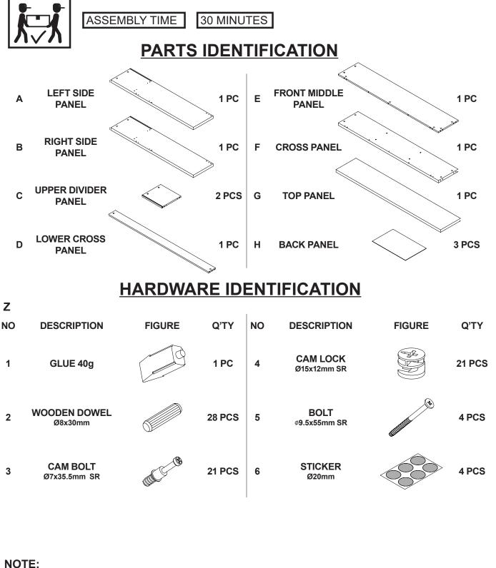
Phillips head screw driver is required in the assembly process; however, manufacturer does not provide this item.
